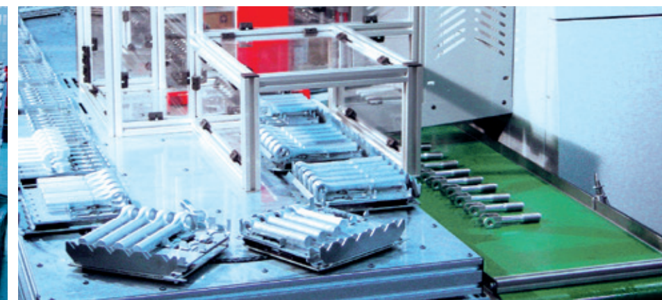
20-station pallet magazine with customer-specific pallets
