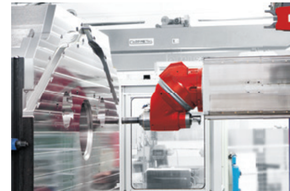
Mechanical machining of a mold by an automatic milling head 6000 rpm
