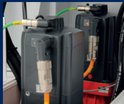
1 X-AXIS KINEMATICS / Dual drive transmission to minimize back-lash and improve accuracy
