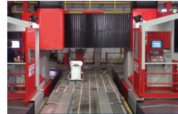
Powermill in the RGM configuration, dedicated to the rails machining
