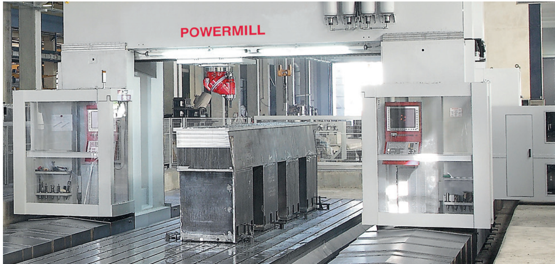
Milling operation on a machine tool structure component
