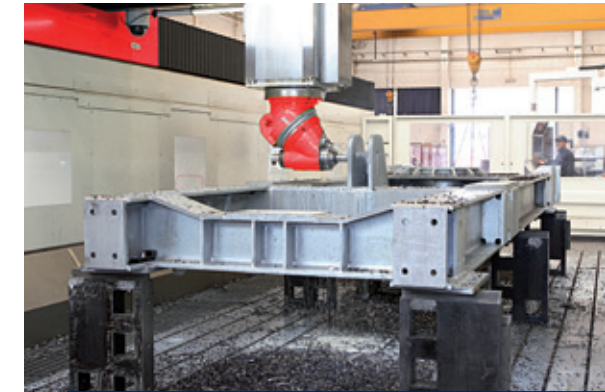
Boring operation on the frame of a CNC machining center for woodworking.
